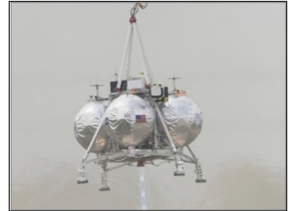
Morpheus Vertical Test Bed: Completed 20 tethered flight tests of Morpheus lander.
