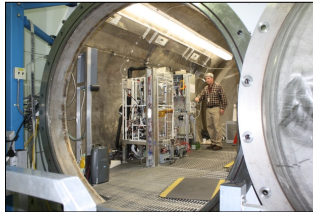
Life Support: Tested ISS-based air revitalization systems to improve reliability.
