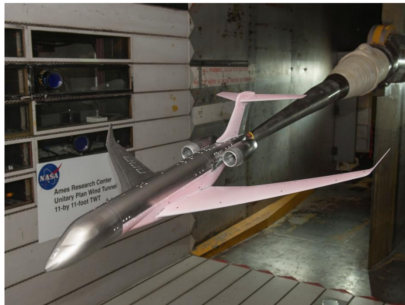
Bombardier Model tests run in Ames Research Center Unitary Plan Wind Tunnel
