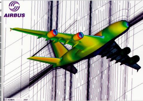
The Aerodynamic Department of Airbus has used ANSYS® ICEM CFD™ software for more than over 10 years to link performance with aerodynamic shape design. AIRBUS
